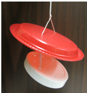
Fig. 6. Example of rain guard attached to lid. Plastic straw spacers between them are optional.
