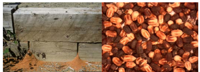
Fig. 8. Comparison of ant and termite frass. Left: carpenter ant frass (sawdust-like) 6 ; right: drywood termite pellets (6-sided, hard, woodlike pellets, ~1mm long) 7 .
